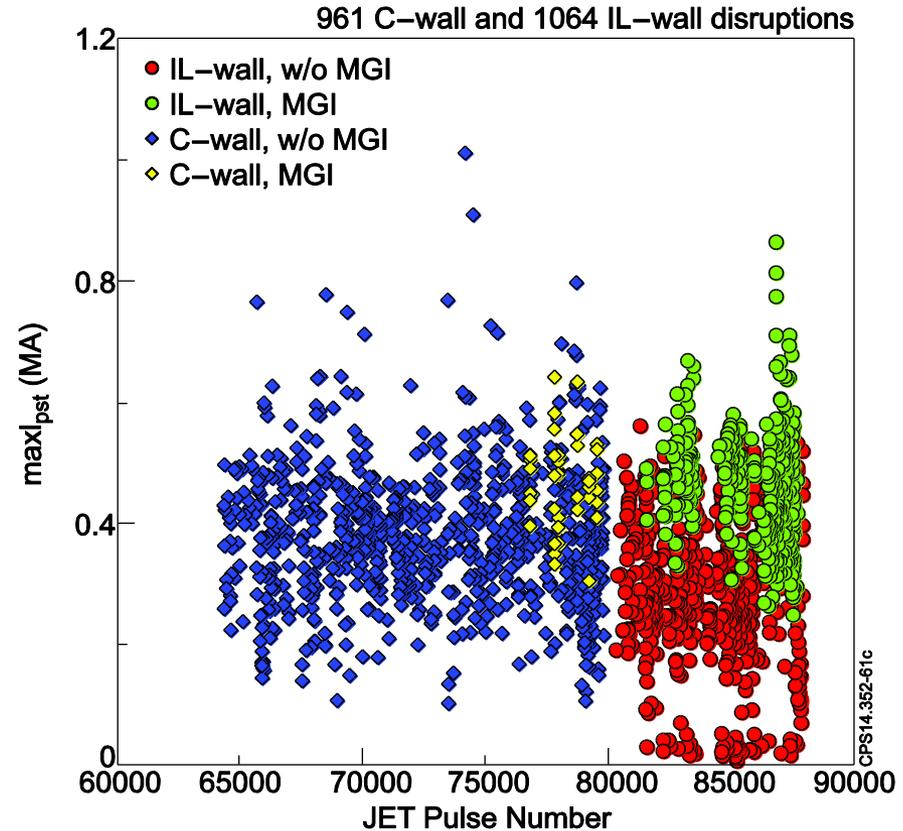
**MGI produces fast plasma current quench and high induced currents, which expose the machine to additional stresses**
