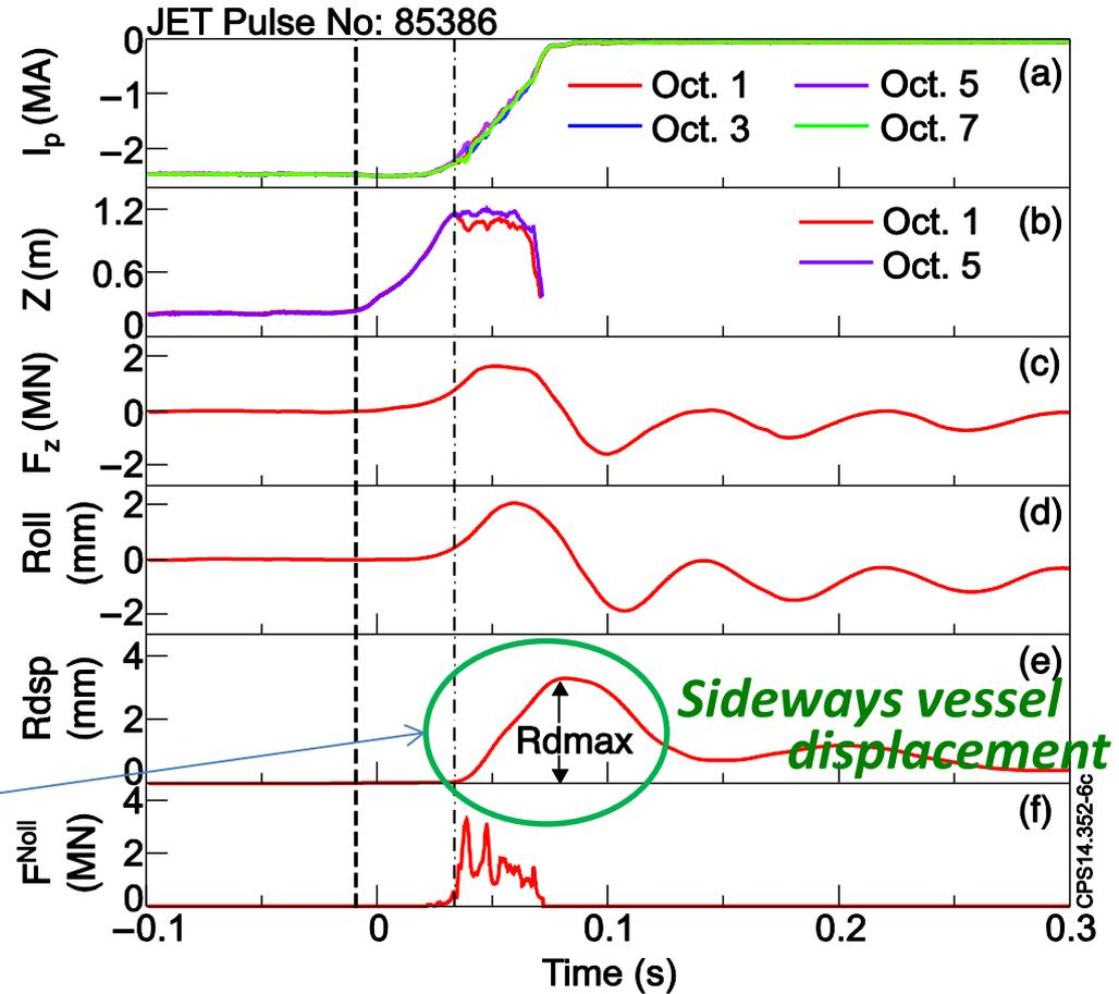
**The JET vessel undergoes a complex, damped oscillation**
