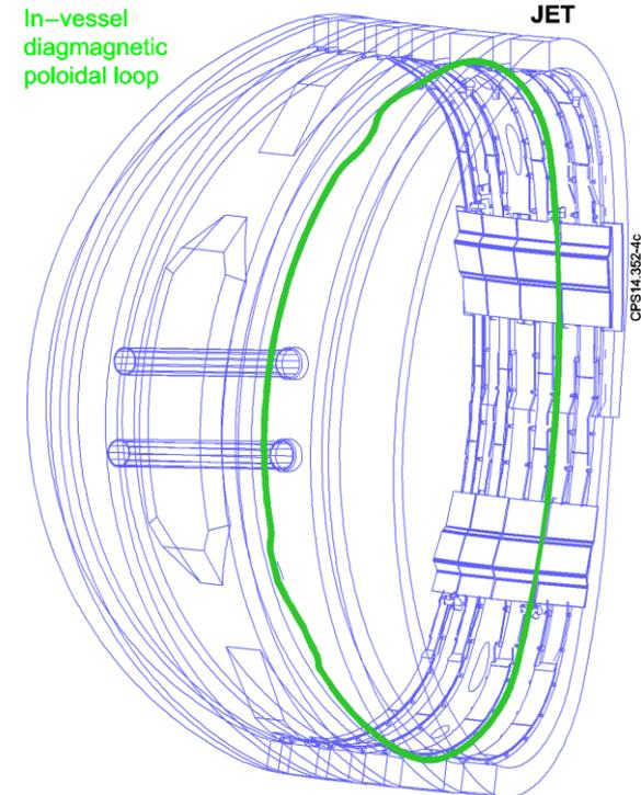
Two **JET** opposite octants equipped with **in-vessel diamagnetic poloidal loops**
