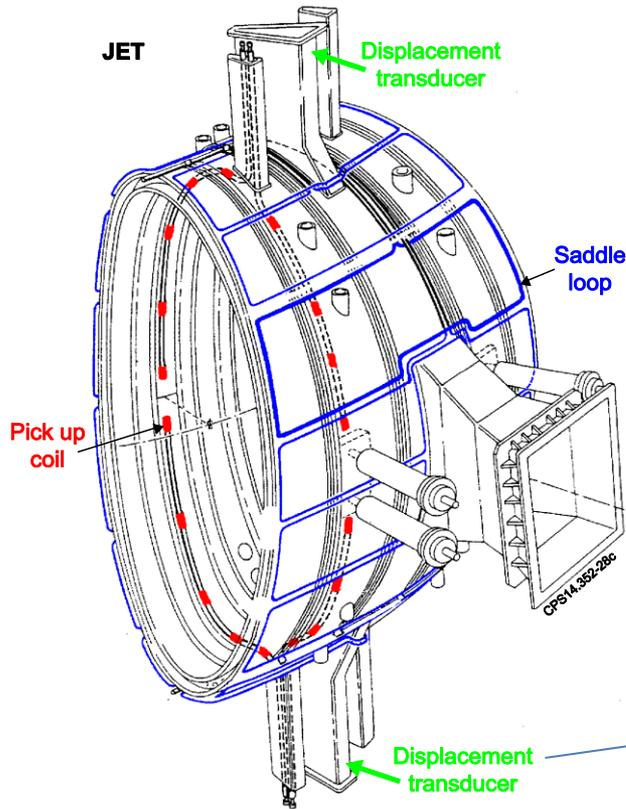
**Transducers** measure radial movement at vertical port of each vessel octant with respect to mechanical structure
