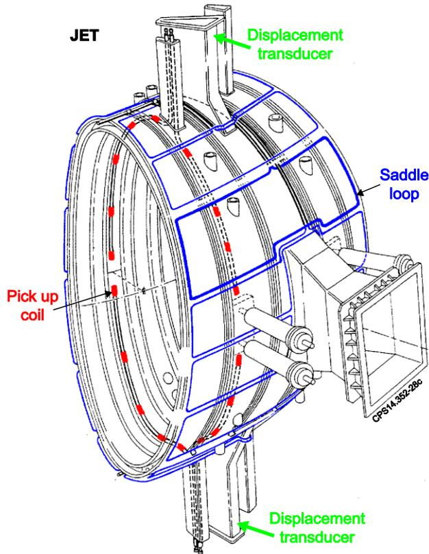
**Transducers measure radial movement of each vessel octant with respect to mechanical structure**
